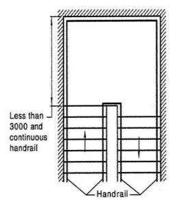
c) Plan of enclosed stair way with landing less than
