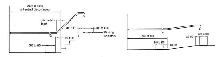
a) Side elevation where bottom landing is greater than 3000m wide and/or has a discontinuous handrail
