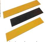
The strips are constructed from a 1.6mm galvanised flat metal strip and coated with a hard wearing UV & chemical resistant 2- part Polyurethane anti-slip coating.
